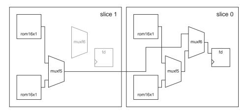
To compose the 6-input LUT with the above placement, we start again by composing the final multiplexer (muxf6) is series with the flip-flip (fd). To specify that they are placed in the same slice, we use the > | > series combinator. In a similar way to before, this is written in Lava as:
