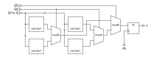
A schematic for the registered 6-input lookup table design is shown in Figure 3.1. This circuit works by addressing four 4-input lookup tables with the least-significant input bits and then selecting between their outputs with the most-significant input bits. The output is registered to provide pipelining when the 6-input lookup table is used to form larger functions.
