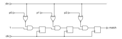
It is possible to implement both the XNOR and AND gates of the repeating structure in a single LUT of the Virtex architecture. The simplest way to describe this combinational logic is therefore to initialise a LUT with the logic function.
